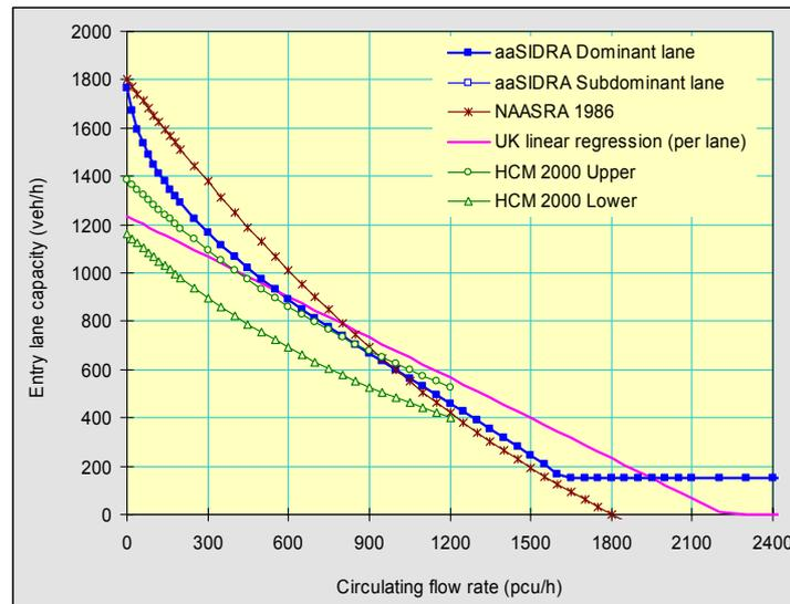
Figure 2 - Model comparison (single-lane roundabout example)
