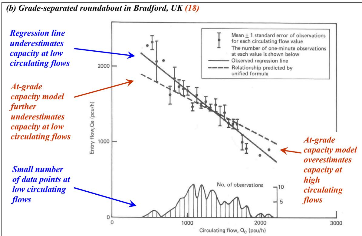
**Figure 3 - Data from roundabout capacity surveys at UK roundabouts**
