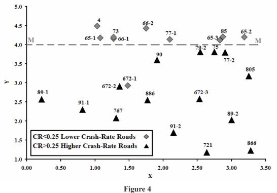
Road Scatter According to Two Dimensions (xi and yi represent the position of highway i based on its infrastructure similarity to other highways)
